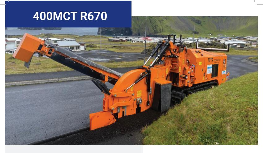
Tesmec 400MCT with R670 is a 11 metric ton-class trencher featuring a 238 Hp (175kW) tier 4/Stage V engine, or a 218 Hp (218 kW) tier 3 engine, designed for telecom and fiber optic projects in urban areas
