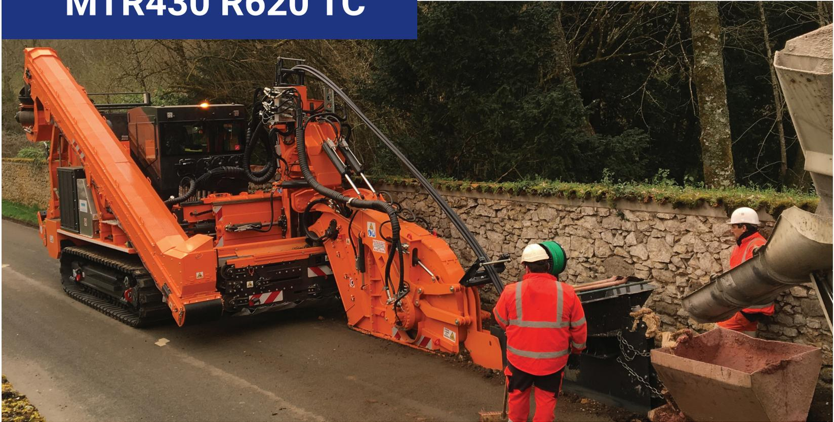
Tesmec MTR430 with R620 is a 30 metric ton-class trencher featuring a 428 HP (315 kW) engine designed to optimise the mechanised laying of networks in rural and urban environments
