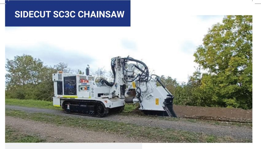
SC3C is a 4 metric ton-class trencher featuring a 98.7 HP (73.6 kW) engine designed for the deployment of fiber optic networks in urban areas
