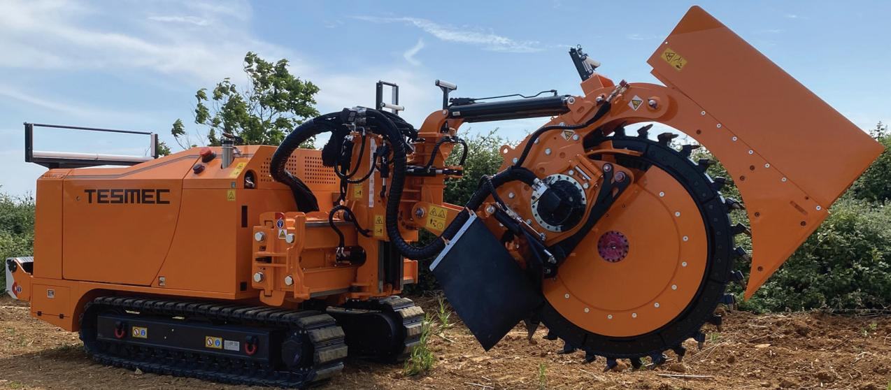
Tesmec 400MCT with RT1100 is a 14 metric ton-class trencher featuring a 238 Hp (175 kW) Tier 4/ Stage V engine, or a 218 Hp (160 kW) Tier 3 engine, designed for telecom and energy cables projects in urban and extra-urban areas
