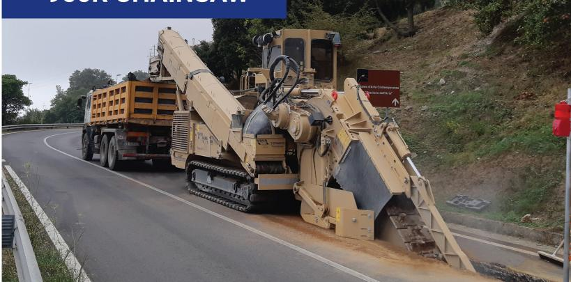
Tesmec 950R Chainsaw is a 25 metric ton-class trencher featuring a 275 HP (205 kW) engine designed for any urban and suburban network: telecom, power lines, gas, water and sewage
