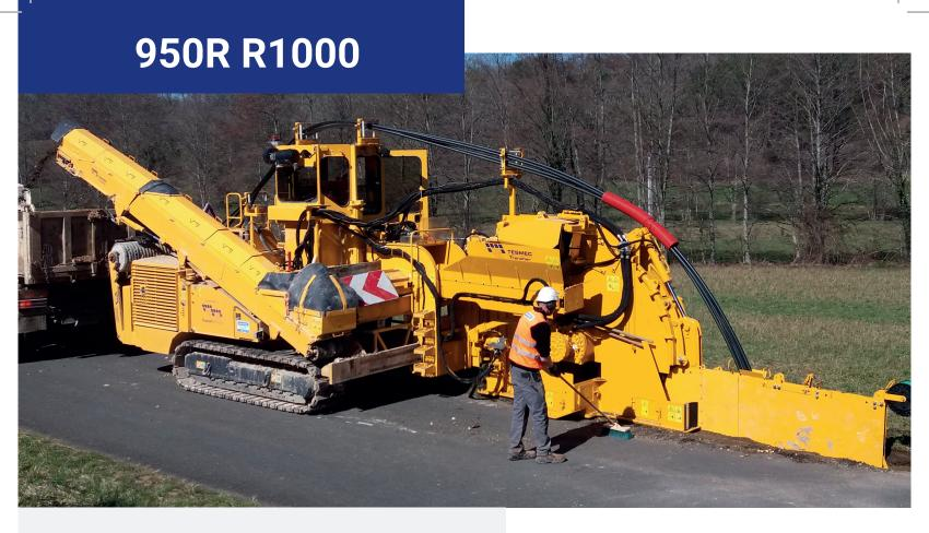
Tesmec 950R R1000 is a 27 metric ton-class trencher featuring with 275 HP (205 kW) engine designed for underground network projects in urban areas
