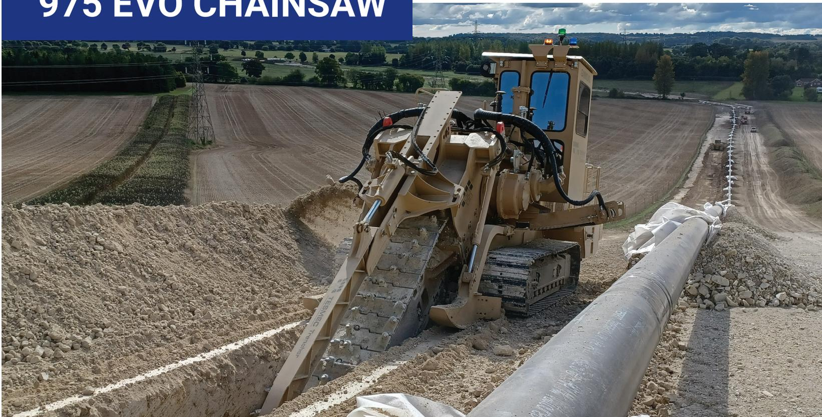
Tesmec 975 EVO Chainsaw is a 40 metric ton-class trencher featuring a 375 HP (285 kW) engine conceived for rock excavation in utilities projects such as fiber optic, electric cables, water conduits, and pipelines
