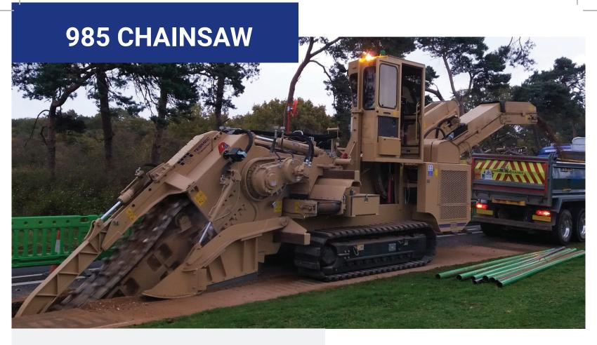
Tesmec 985 Chainsaw is a 40 metric ton-class trencher equipped with a 375 HP (280 kW) engine conceived for all ranges of customers, from highway contructors to pipeline contractors, working on projects where space is one of the main issues
