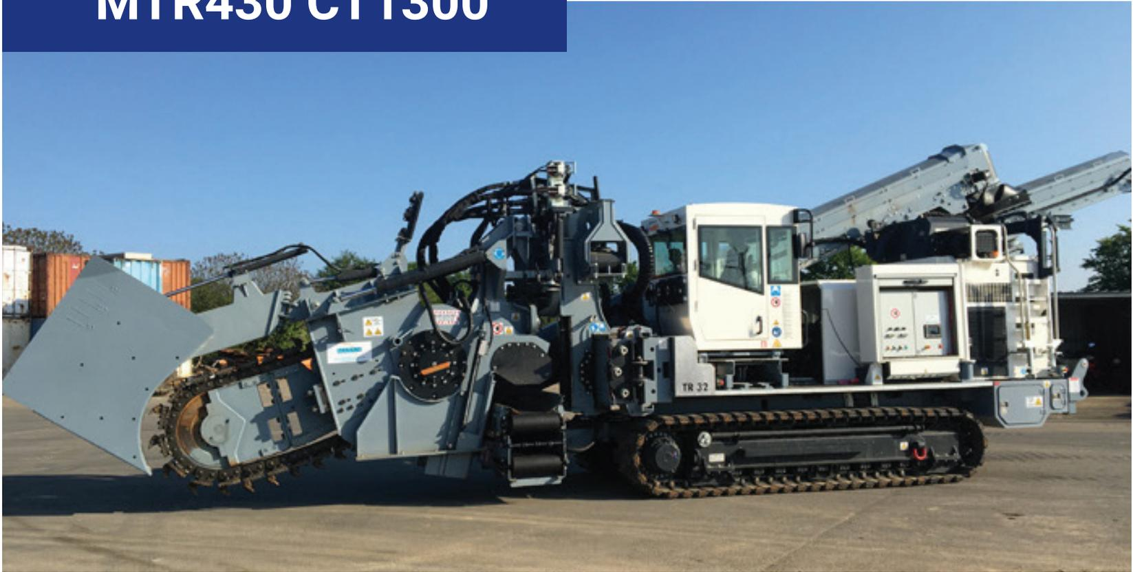
Tesmec MTR430 with CT1300 is a 33 metric ton-class trencher featuring a 428 HP (315 kW) engine designed to optimise the mechanized laying of networks in rural and urban environments
