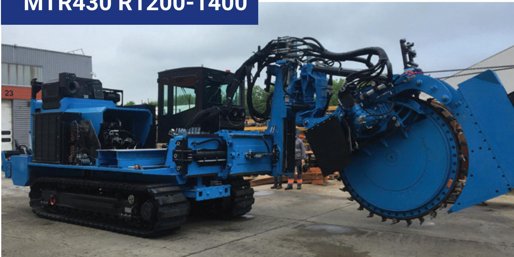
Tesmec MTR430 with R1200 or R1400 is a 30 metric ton-class trencher featuring a 428 HP (315 kW) engine designed to optimise the mechanized laying of networks in rural and urban environments
