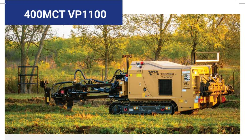
Tesmec 400MCT with VP1100 vibratory plow is a 10 metric ton-class trencher featuring a 238 Hp (175kW) tier 4 engine/Stage V, or a 218 Hp (218 kW) tier 3 engine, designed for telecom and energy cable projects in rural areas
