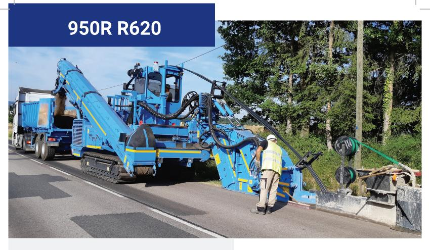
Tesmec 950R R620 is a 25 metric ton-class trencher featuring a 275 HP (205kW) engine designed for telecom and fiber optic projects in urban areas
