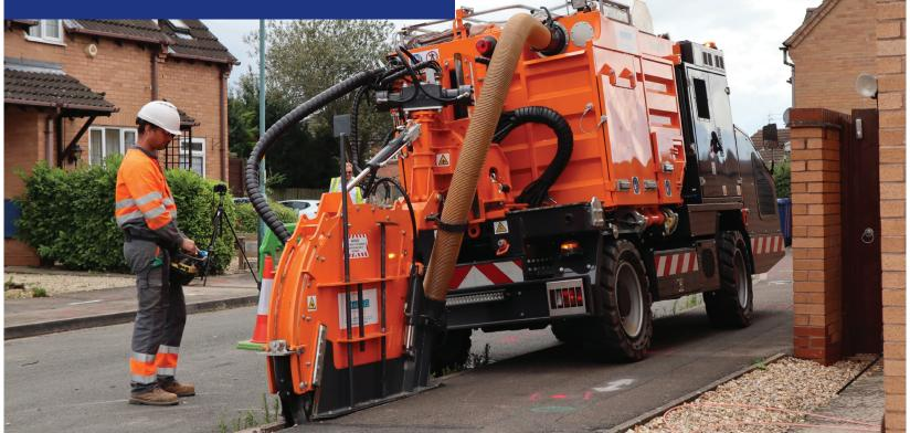
Tesmec CityCleanfast is a 10 metric ton-class trencher featuring a 142 HP (105 kW) engine conceived for a clean and fast deployment of fiber optic in urban environments.
