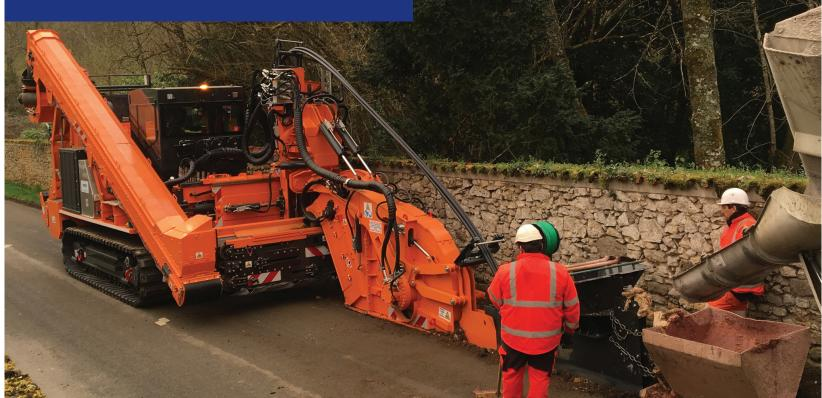
Tesmec MTR430 with R620 is a 30 metric ton-class trencher featuring a 428 HP (315 kW) engine designed to optimise the mechanised laying of networks in rural and urban environments
