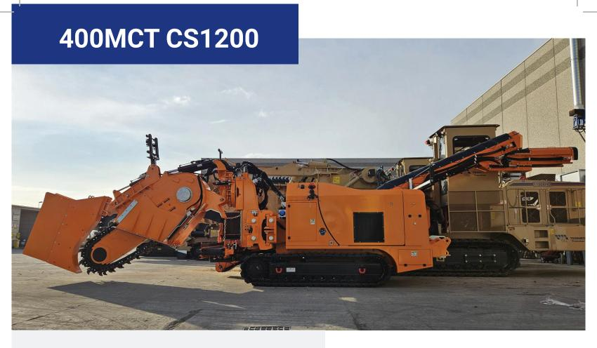
Tesmec 400MCT with CS1200 is a 15 metric ton-class trencher featuring a 238 Hp (175 kW) tier 4 engine/ Stage V, or a 218 Hp (160 kW) tier 3 engine, designed for telecom and energy cables projects in urban and extra-urban areas
