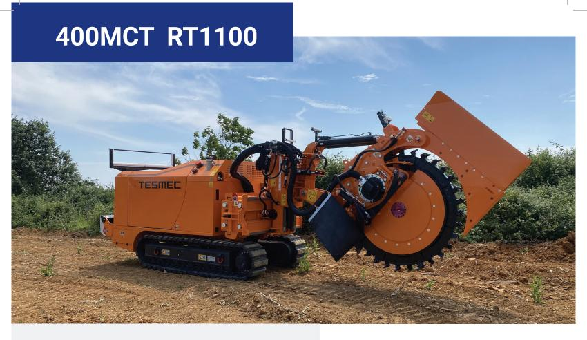
Tesmec 400MCT with RT1100 is a 14 metric tonclass trencher featuring a 238 Hp (175 kW) Tier 4/ Stage V engine, or a 218 Hp (160 kW) Tier 3 engine, designed for telecom and energy cables projects in urban and extra-urban areas
