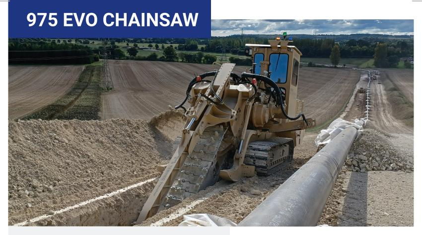
Tesmec 975 EVO Chainsaw is a 40 metric ton-class trencher featuring a 375 HP (285 kW) engine conceived for rock excavation in utilities projects such as fiber optic, electric cables, water conduits, and pipelines
