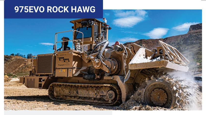
Tesmec 975 EVO Rock Hawg is a 44 metric ton-class surface miner featuring a 375 HP (280 kW) engine employed in bulk excavations, tunneling projects and continuous surface mining
