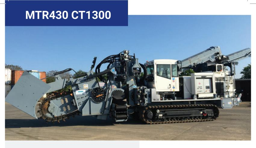
Tesmec MTR430 with CT1300 is a 33 metric ton-class trencher featuring a 428 HP (315 kW) engine designed to optimise the mechanized laying of networks in rural and urban environments
