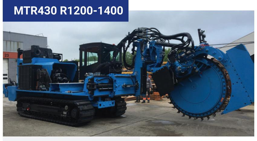
Tesmec MTR430 with R1200 or R1400 is a 30 metric ton-class trencher featuring a 428 HP (315 kW) engine designed to optimise the mechanized laying of networks in rural and urban environments
