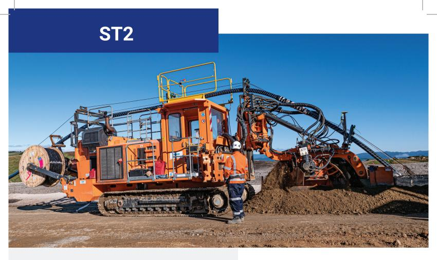
Tesmec ST2 is a 25-30 metric ton-class trencher featuring a 510 HP (375 kW) Tier 4/Stage V engine, or a 536 HP (394 kW) Tier 3 engine, designed to allow the simultaneous trenching and mechanical laying for the deployment of networks in rural environments and rocky grounds
