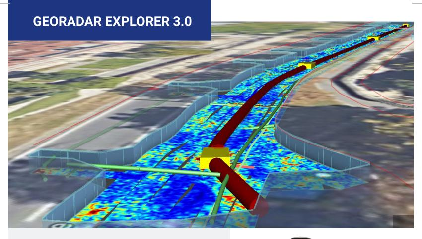
Tesmec Georadar Explorer 3.0 is a Ground Probing Radar - GPR - which detects underground utilities, optimizing trenching and laying operations.
