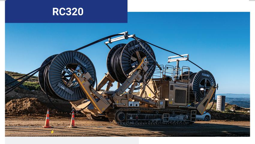
Tesmec RC320 is a 44 metric ton-class reel carrier featuring a 250 Hp (186kW) Tier 3 engine, or a 275 HP (205 kW) tier 4/Stage V designed to carrying and unrolling cables or pipes. It is conceived for energy cable projects.
