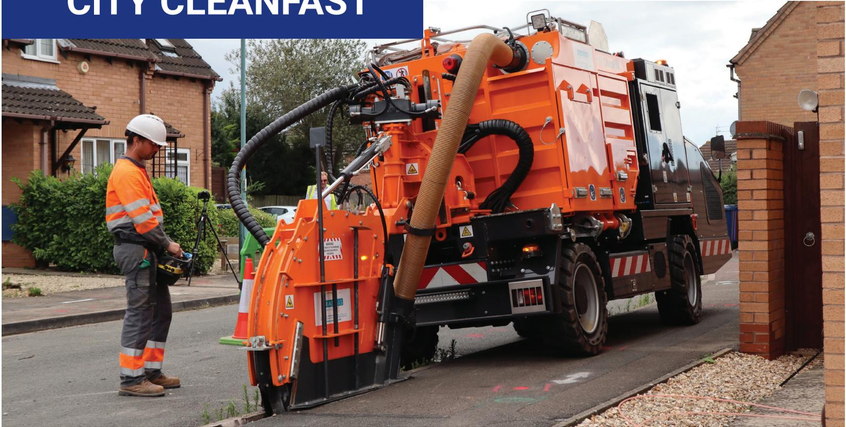
Tesmec CityCleanfast is a 10 metric ton-class trencher featuring a 142 HP (105 kW) engine conceived for a clean and fast deployment of fiber optic in urban environments.
